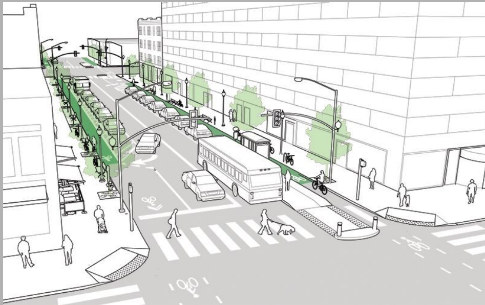
Image above is an example of a complete street. Image by NACTO
