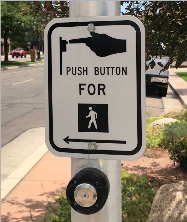
Pedestrian Activated Signal such as this one allows the pedestrian to activate the signal to cross.
